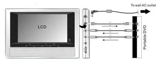
Note: the AC adapter must connect to the extra screen or it will not have power.
